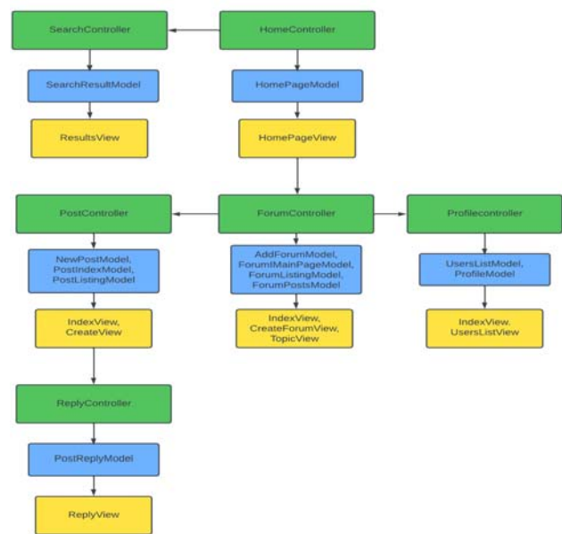
Figure 2 – Graphical model of the MVC logical structure of the ForumModel web forum
