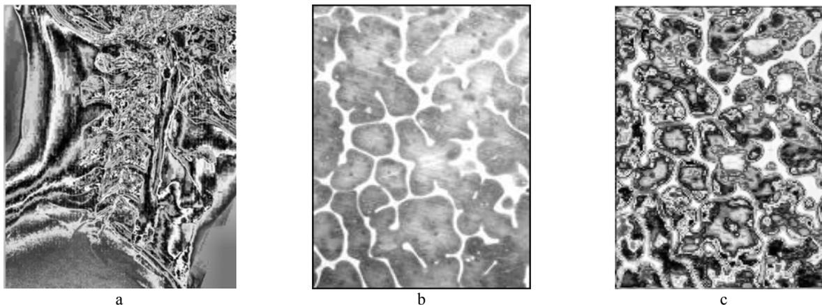
Figure 5 – Image segmentation: a – segmentation of the X-ray image from Figure 2 c; c – segmentation of the optoelectronic metallographic image from Figure 5 b
