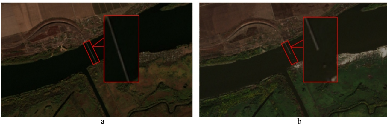
Figure 3 – Multi-temporal Sentinel-2 images of the Antonivsky Railway Bridge: a – 2021 before destruction; b – 2023 after destruction
