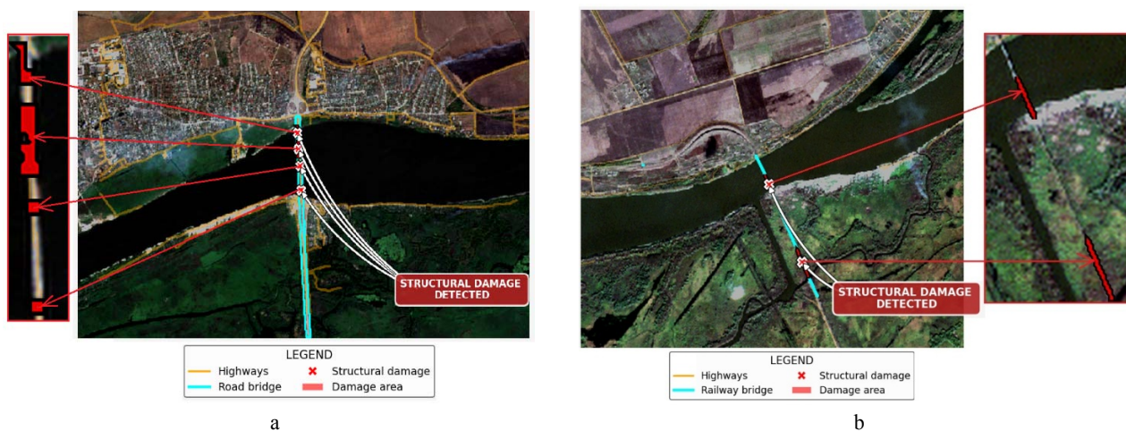
Figure 8 – The result of the proposed neural network method for damage detection in 2023: a – Antonivsky automobile bridge; b – Antonivsky railway bridge
