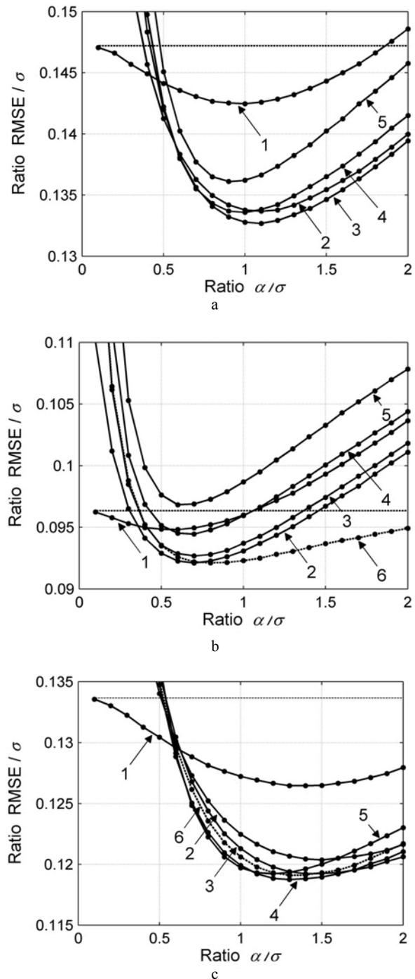
Figure 2 – RMSE/ $\sigma$  ratio vs  $\alpha/\sigma$  ratio for the constant signal distorted by the (a) Cauchy noise, (b) mixture of Cauchy and Laplacian noise, and (c) mixture of Cauchy and Gaussian noise
