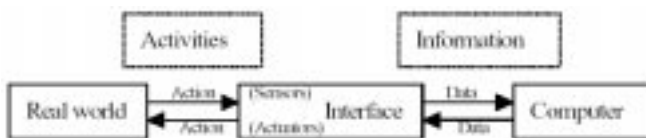
Figure 1 - Block diagram of signal processing on a humanoid designed by traditional concept (Here, the data are transferred through media)
