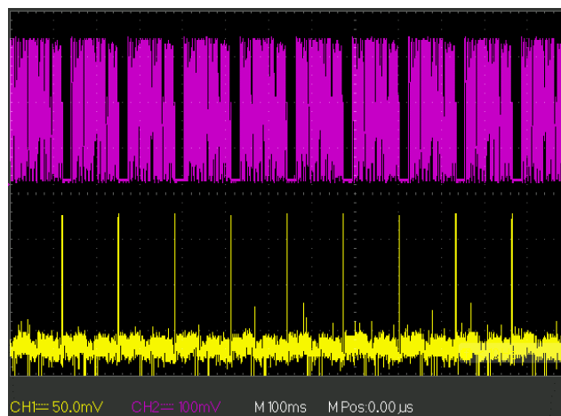
Figure 8 – The oscillograms of the voltage at the input and output of the optimal processing block of the LFM signal for command number one
