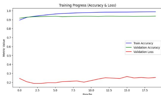
Figure 6 – Training process after performing K-Fold cross-validation for CNN, LSTM, and the Attention mechanism: changes in accuracy and loss
